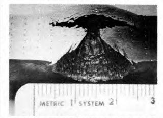
ACTUAL DEFORMATION of steel plate by nylon ball. The ball was vaporized by the impact.
